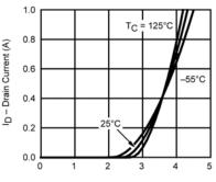
V<sub>GS</sub> – Gate-to-Source Voltage (V)
